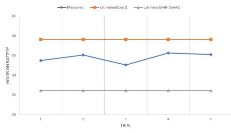
Battery trial results: Measured time on battery verses ideal battery life with and without a safety factor of 1.5.
