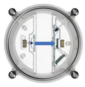
The white LED emits light through the water to the TCS34725 RGB Sensor to collect the color and turbidity reading
